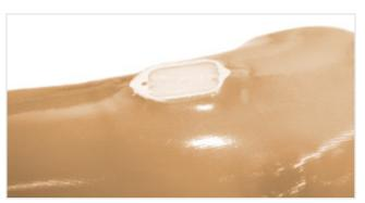
4. Once the lamination procedure is complete, the outer surface over the blank is ground away to the level of the inner socket lamination blank.
