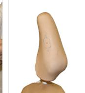
2. Apply nylon stockinette to the cast to act as a wick during the vacuum forming process.
