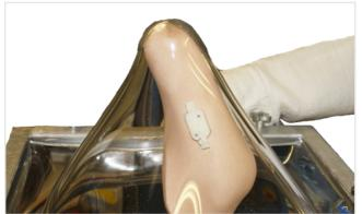
6. Heat thermoplastic material in an oven as per manufacturer's guidelines and once ready drape the material over the cast taking care to ensure any wrinkles are pulled beyond the proximal trim. For more information on electrode fabrication please contact a Steeper product manager or our customer services team who will be happy to assist with your enquiry.
