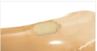
5. Remove the inner socket lamination blank completely. Fit the outer socket lamination blank ensuring that the pip is situated proximally. Proceed to fabricate the forearm in the usual manner.
