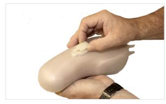
9. Insert the outer socket vacuum blank (from vacuum kit E25591) with the tongue pointing towards the wrist and proceed to fabricate the forearm.
