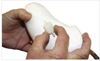
1. Identify the position of the electrodes on the cast and check this area is completely flat to ensure a close fit of the inner socket lamination blank (from lamination kit E25590).
