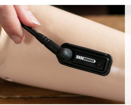
The S-Charge System is a user friendly, powerful internal battery system, with an OLED display and a magnetic charger which can all be installed into a prosthesis. This allows the user to easily activate, deactivate, and charge their prosthesis while confidently monitoring the power status during the day.
