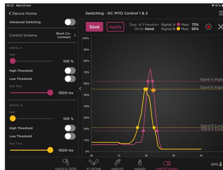
Each degree of freedom will have a main display screen to view the live action of the device being controlled. Configurations will vary based on the control method that is set up: **Myo Sites**, **a Linear Transducer**, **Physical Switches** or **Pattern Recognition** (example: 2-site Myo).
