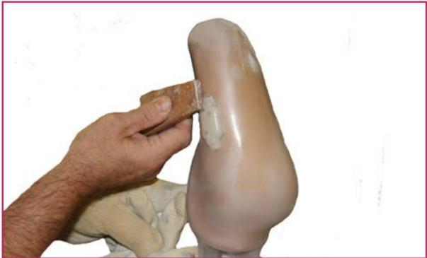
8. Once the material has cooled, the outer surface over the blank is ground away to the level of the electrode mounting bracket blanks. Remove the inner socket vacuum blank.
