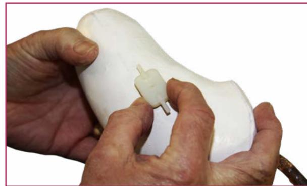
2. Apply a PVA sheet to the cast, with the gloss side in, ensuring there are no wrinkles within the socket area, and apply the vacuum. Attach the inner socket lamination blank using the attached double sided tape and feed 2 small pieces of dacron felt under the legs of the blank.
