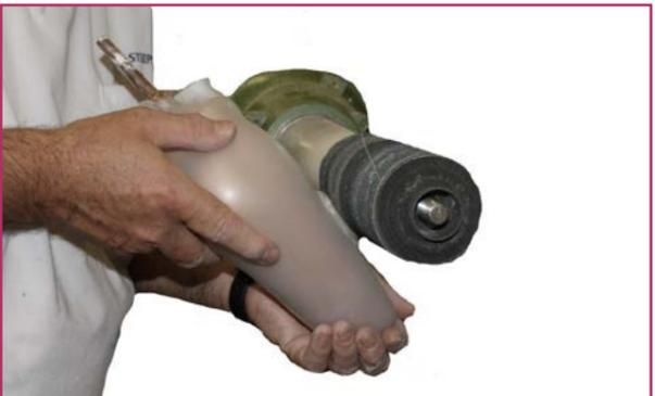
9. Insert the outer socket vacuum blank (from vacuum kit E25591) with the tongue pointing towards the wrist and proceed to fabricate the forearm.
