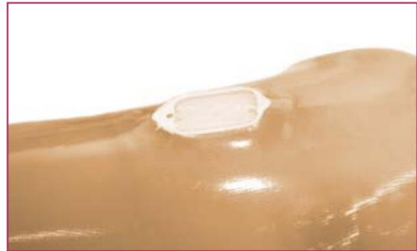
5. Remove the inner socket lamination blank completely. Fit the outer socket lamination blank ensuring that the pip is situated proximally. Proceed to fabricate the forearm in the usual manner.
