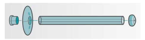
Assemble the drying stand as shown by inserting the tube through the disc, then onto the base. Finally, place the cap on top of the tube. The drying stand may be shortened by trimming the tube before placing onto the base.
