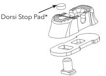
FIGURE 5B: Seattle Kinetic Edge - Dorsi stop inserted into pad spacer. er, bumper and dorsi stop pad \*This is a standard component of the Seattle Kinetic Edge (SKF300, SKF301, SKF303). When refurbishing all other Seattle Kinetic Foot feet, this component is optional.
