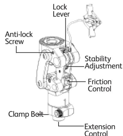
**FIGURE 2:** Child's Play Knee with Manual Lock adjustments
