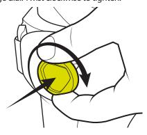
7 Pull up on dial to release tension: Lift Velco tab to release.
