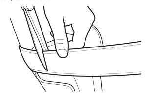
6 Push to engage dial: Twist clockwise to tighten.
