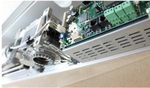
To provide additional safety, two sensors are installed on the door opener. The large sensor fits onto the opening side of the door and the small sensors are placed on the closing side of the door, ensuring that the door does not close on the residents as they pass through.
